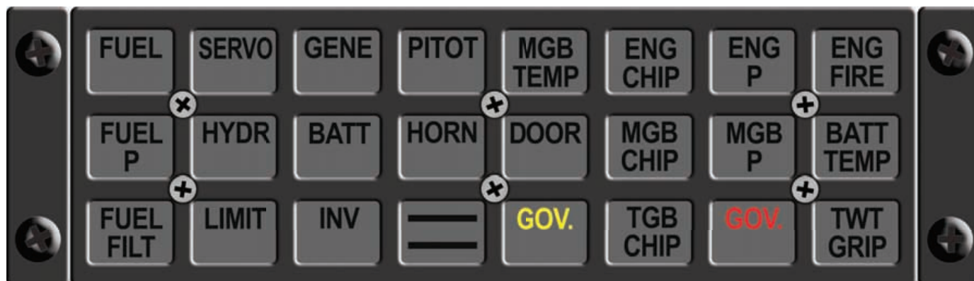
AS350B3 Governor Failure Indication.
